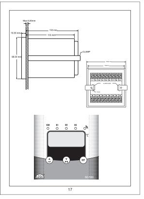
**Controller**: Controller should be installed in a place protected by vibration, water and corrosive gasses and where ambient temperature does not exceed the values specified in the technical data.
